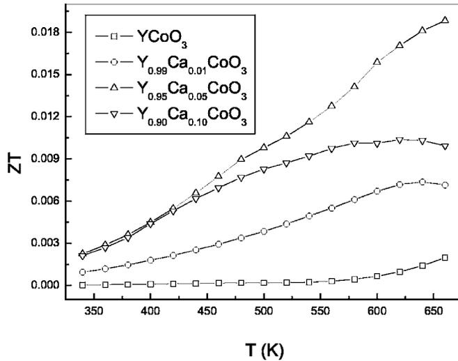
FIG. 8. Dimensionless figure of merit  $ZT$  as a function of temperature  $T$  for  $Y_{1-x}Ca_xCoO_3$  ( $x=0, 0.01, 0.05, 0.1$ ).
