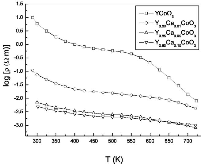
FIG. 1. Electrical resistivity  $\rho$  as a function of temperature  $T$  for  $Y_{1-x}Ca_xCoO_3$  ( $x=0, 0.01, 0.05, 0.1$ ).
