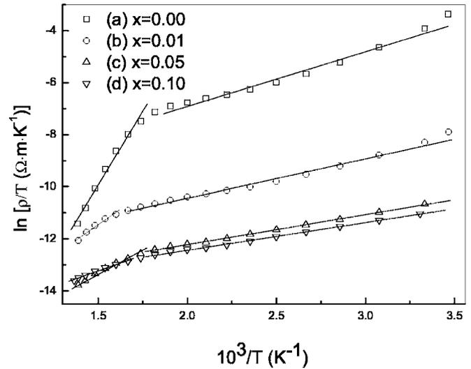
FIG. 2. Plot of  $\ln(\rho/T)$  vs  $1/T$  for  $Y_{1-x}Ca_xCoO_3$  ( $x=0, 0.01, 0.05, 0.1$ ) with (a)  $x=0$ , (b)  $x=0.01$ , (c)  $x=0.05$ , and (d)  $x=0.1$ . The solid lines are the best fit of the experimental data to formula (2).
