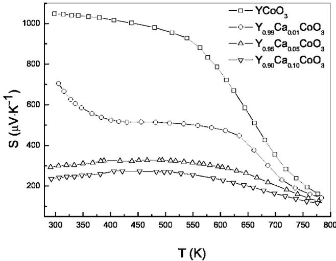
FIG. 5. Seebeck coefficient  $S$  as a function of temperature  $T$  for  $Y_{1-x}Ca_xCoO_3$  ( $x=0, 0.01, 0.05, 0.1$ ).
