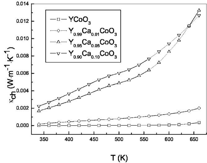
FIG. 7. Carrier thermal conductivity  $\kappa_{ch}$  as a function of temperature  $T$  for  $Y_{1-x}Ca_xCoO_3$  ( $x=0, 0.01, 0.05, 0.1$ ).
