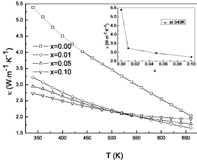
FIG. 6. Thermal conductivity  $\kappa$  as a function of temperature  $T$  for  $Y_{1-x}Ca_xCoO_3$  ( $x=0, 0.01, 0.05, 0.1$ ). The inset shows the plot of  $\kappa$  vs Ca content  $x$  at 340 K for  $Y_{1-x}Ca_xCoO_3$ .
