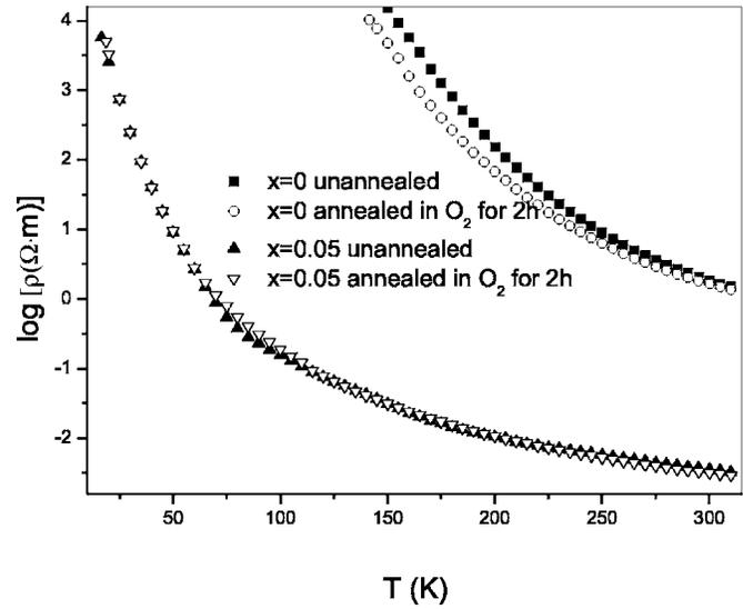
FIG. 4. Typical plots of  $\log \rho$  vs temperature  $T$  for the  $Y_{1-x}Ca_xCoO_3$  with  $x=0$  and 0.05 unannealed and annealed in oxygen.
