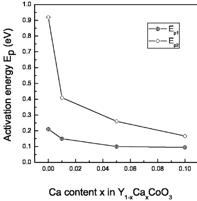
FIG. 3. Activation energy  $E_p$  vs Ca content of doping  $x$  in low-temperature ( $E_{p1}$ ) and high-temperature ( $E_{p2}$ ) regions for  $Y_{1-x}Ca_xCoO_3$  ( $x = 0, 0.01, 0.05, 0.1$ ).
